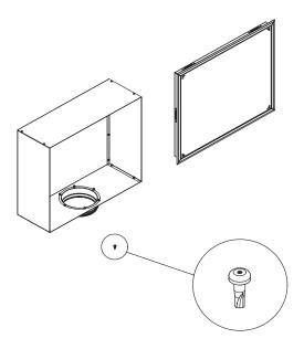
Tool for loosening the perforated face plate from the nozzle plate
